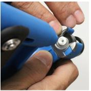
Remove the red plastic clip by pulling it outward. Be careful as the metal cutter above the clip is very sharp. Ensure the applicator is loaded with an unused green punch (if the red plunger is visible, the punch is used and should be replaced with one that is unused).
