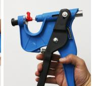
Rotate the black chamber to lock the punch into the device. Carefully squeeze the applicator handles together, guiding the punch tip into place if necessary. When the gun bolt rests flush against the red plastic clip, release the handle.
