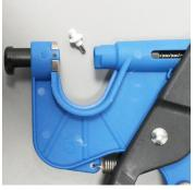
Reopen the chamber and remove the punch from the applicator. Check that sampling has been successful (red plunger is visible, sample is in fluid in punch). Remove the used cutter from the applicator by pulling the handles apart. Discard carefully as the cutter is very sharp.
